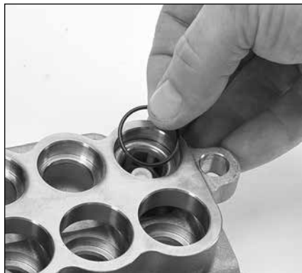
2.20 Lubricate and install valve seat O-ring into the inlet valve bore.
