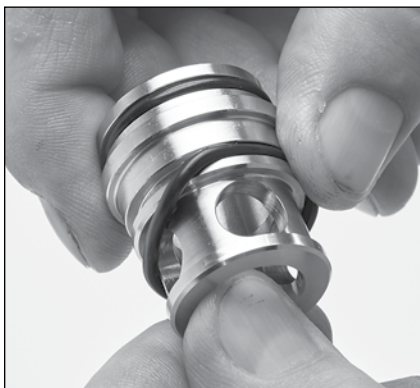
1.44 Replace front discharge valve adapter O-ring with new one from seal kit and apply a lubricant to outside surface.
