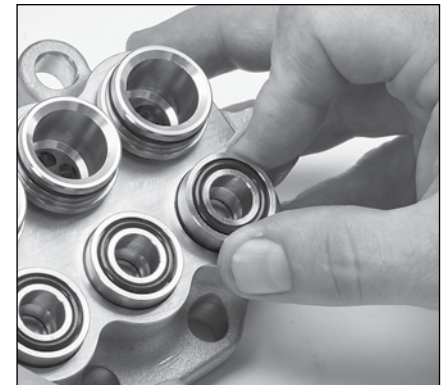
1.48 With larger O-ring side facing down, install inlet valve adapter into inlet manifold bore. Twist and press into place.
