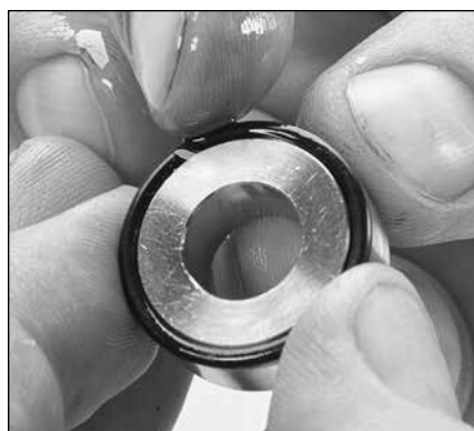
2.25 Replace front inlet valve adapter O-ring with new one from seal kit and apply a lubricant to outside surface.
