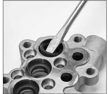
1.12 Use a flat tip screwdriver to pry the high-pressure seals upward and remove.
