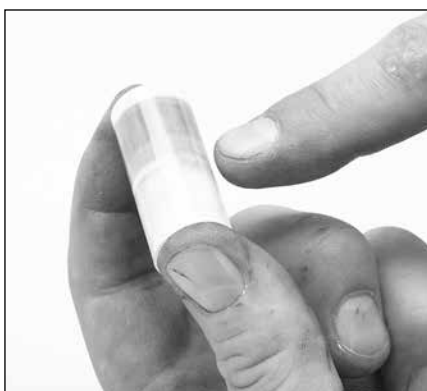
1.22 Inspect ceramic plunger for cracks and scoring to the surface. Clean with a wire-wheel brush if necessary.
