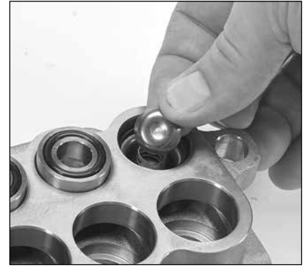
2.15 Remove the inlet valve. Inspect tapered surface of the valve for wear, pitting or damage.
