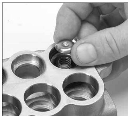
2.22 Place the valve onto the spring with concave side facing down.
