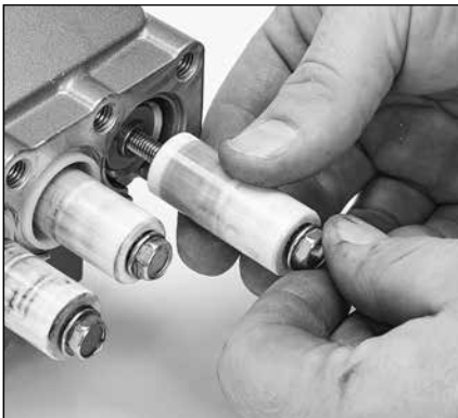
1.30 Thread plunger assembly into plunger rod by hand, and torque to 55 in-lbs, 4.6 ft-lbs or 6.2 Nm.
