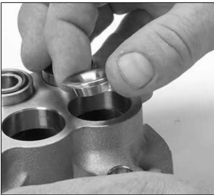
2.31 Place the valve seat onto the valve with the tapered surface facing down.
