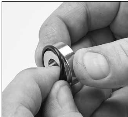
1.17 Remove the front inlet valve adapter O-ring. Inspect O-ring for cuts, nicks or damage.
