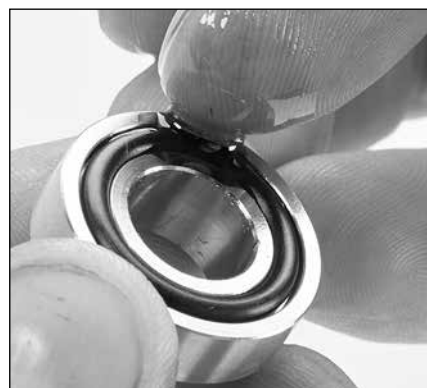
2.24 Replace rear inlet valve adapter O-ring with new one from seal kit and apply a lubricant to outside surface.
