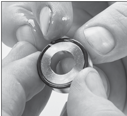
1.47 Replace front inlet valve adapter O-ring with new one from seal kit and apply a lubricant to outside surface.
