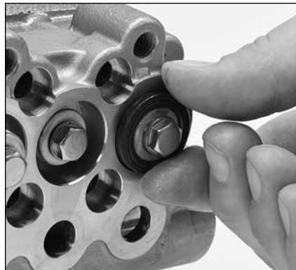
1.39 One side of the high-pressure seal has a groove. Install groove side facing out and press into place.
