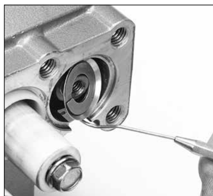
1.23 Use a pick to remove keyhole washer and barrier slinger located behind the plunger. Inspect for damage.
