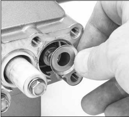
1.24 Install barrier slinger with dish side facing away from crankcase.
