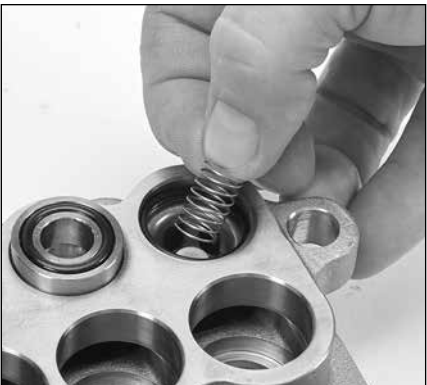
2.16 Remove the spring. Check for proper tension or any damage.
