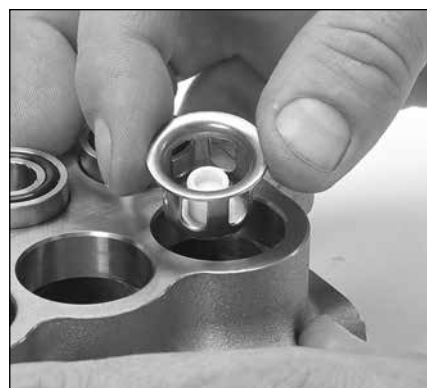
2.27 Install spring retainer with white notch facing down into the discharge valve bore.
