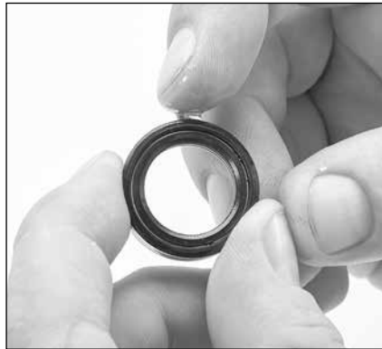
1.33 Apply a lubricant to the outside surface of the low-pressure seals.
