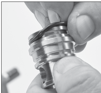
1.43 Replace rear discharge valve adapter O-ring with new one from seal kit and apply a lubricant to outside surface.
