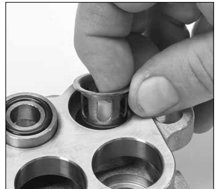
2.18 Remove the inlet spring retainer. Inspect for cracks, excessive wear or damage.
