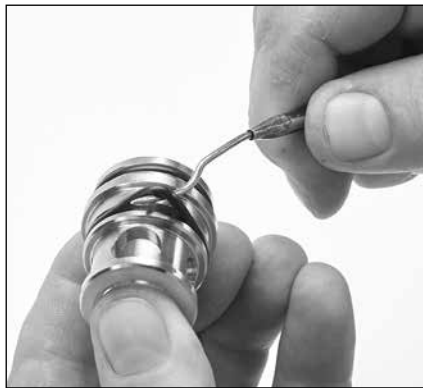
1.14 Using a pick, remove the front discharge valve adapter O-ring. Inspect O-ring for cuts, nicks or damage.
