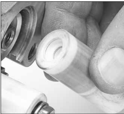
1.27 Look for stepped side of plunger. This side goes towards the pump crankcase.
