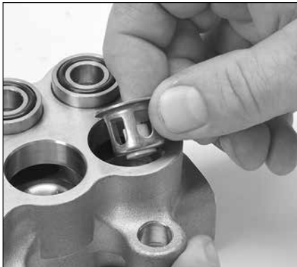
2.10 Remove the discharge spring retainer. Inspect for cracks, excessive wear or damage.
