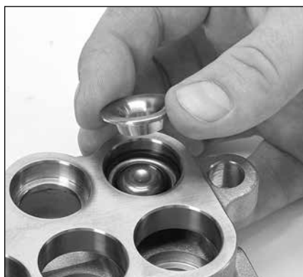
2.23 Place the valve seat onto the valve with the tapered surface facing down.
