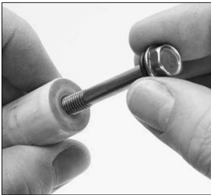
1.28 Insert plunger retainer with gasket into non-stepped side of plunger.
