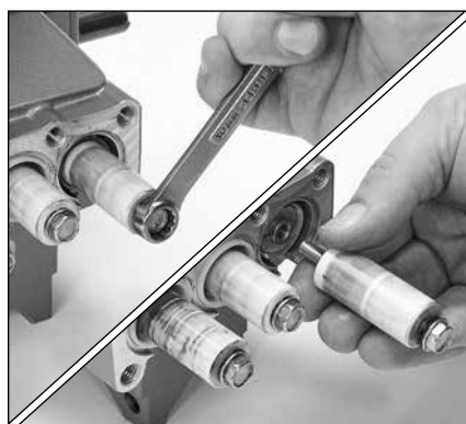
1.20 Using a 10 mm combination wrench, loosen and remove the plunger retainer and plunger.
