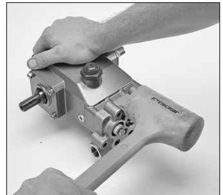
1.37 Use a rubber mallet to tap manifold on the rest of the way.
