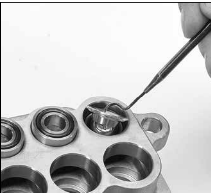
2.14 Using a pick, remove the inlet valve seat. Inspect tapered surface of the valve seat for wear, pitting or damage.
