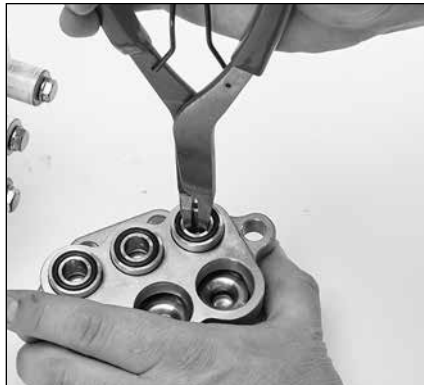
2.11 Using a reverse pliers, grasp the inside diameter of the inlet valve adapter. Remove with a twisting motion.
