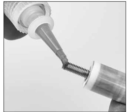
1.29 Place a drop of Loctite® 242® on the threaded end of the plunger rod.
