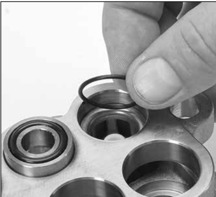
2.17 Remove the valve seat O-ring. Inspect O-ring for cuts, nicks or damage.
