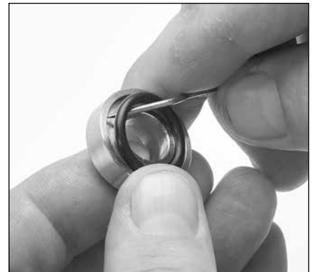
1.18 Using a pick, remove the rear inlet valve adapter O-ring. Inspect O-ring for cuts, nicks or damage.
