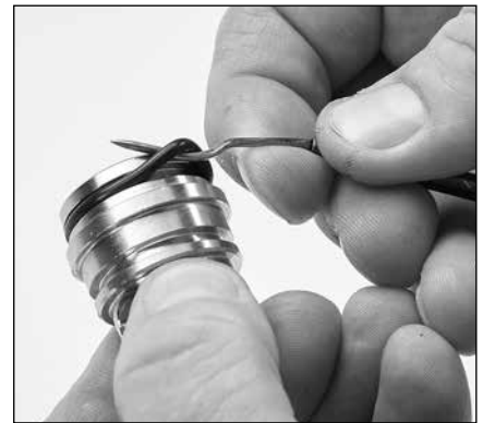
1.15 Using a pick, remove the rear discharge valve adapter O-ring. Inspect O-ring for cuts, nicks or damage.
