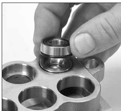
2.26 With larger O-ring side facing down, install inlet valve adapter into inlet manifold bore. Twist and press into place.
