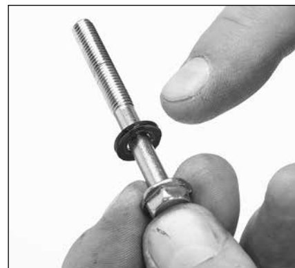
1.21 Remove and inspect plunger retainer gasket.
