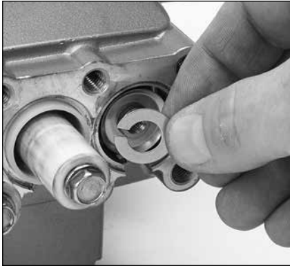
1.25 Install keyhole washer. The slot can face any direction.
