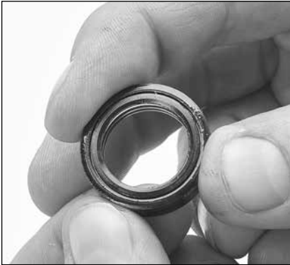
1.10 Inspect the inside diameter of the low-pressure seals for wear or damage.
