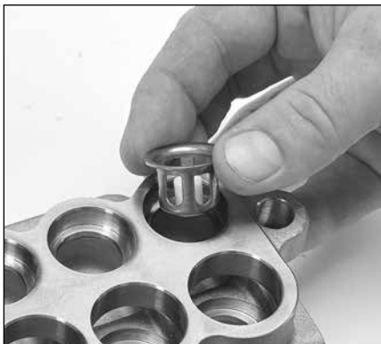
2.19 Install spring retainer with white notch facing down into the inlet valve bore.
