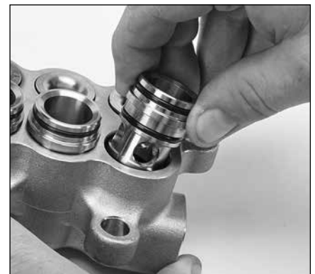
2.33 With smaller side facing down, install discharge valve adapter into discharge manifold bore. Twist and press into place.
