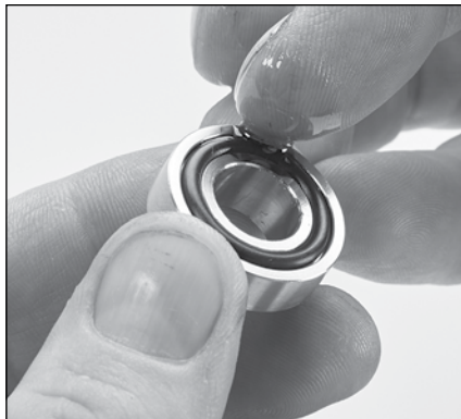
1.46 Replace rear inlet valve adapter O-ring with new one from seal kit and apply a lubricant to outside surface.
