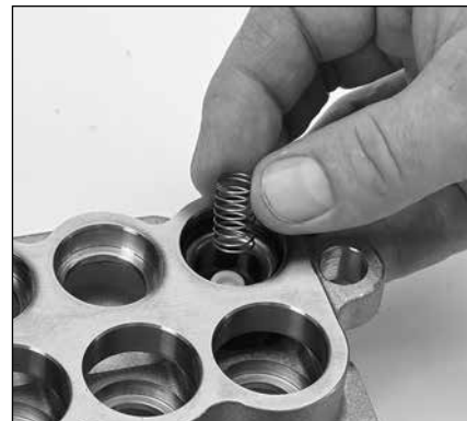
2.21 Place the spring onto the guide in the spring retainer.
