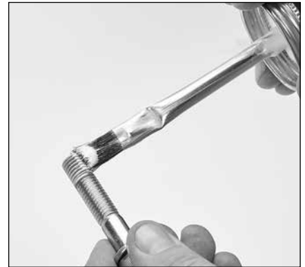
1.51 Apply anti-seize to the six (6) HSH screws.
