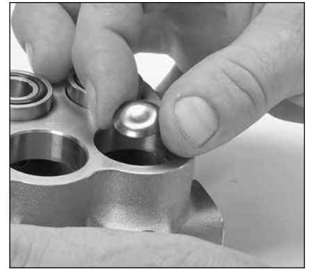
2.30 Place the valve onto the spring with concave side facing down.
