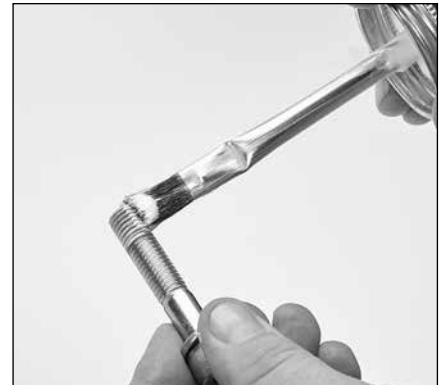
2.36 Apply anti-seize to the six (6) HSH screws.
