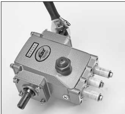
1.35 Rotate crankshaft so outside two plungers are even at furthest distance from crankcase.
