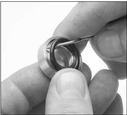
2.13 Using a pick, remove the rear inlet valve adapter O-ring. Inspect O-ring for cuts, nicks or damage.
