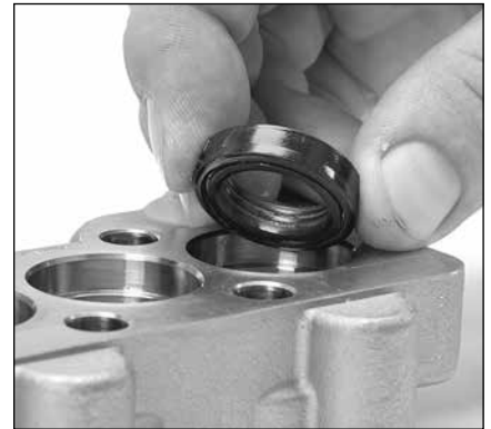
1.34 One side of the low-pressure seal has a groove and spring. Install groove side facing down and press into place.
