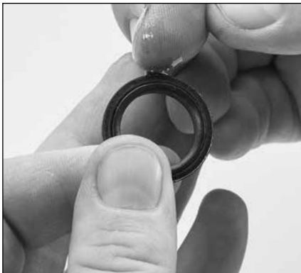
1.38 Apply a lubricant to the outside surface of the high-pressure seals.
