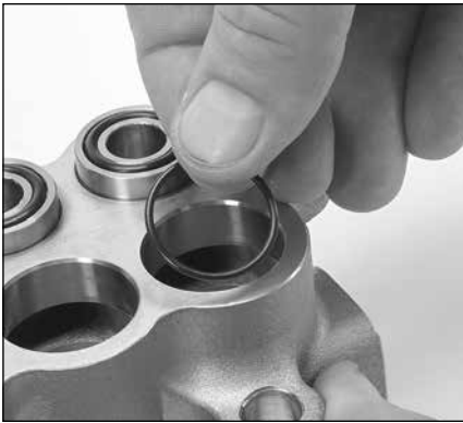
2.28 Lubricate and install valve seat O-ring into the discharge valve bore.
