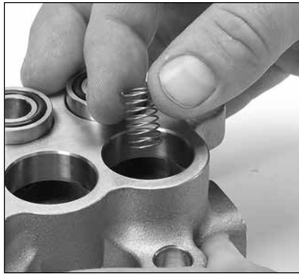
2.29 Place the spring onto the guide in the spring retainer.
