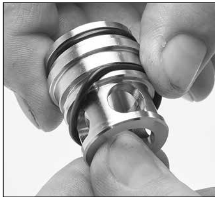
2.32 Replace front discharge valve adapter O-ring with new one from seal kit and apply a lubricant to outside surface.
