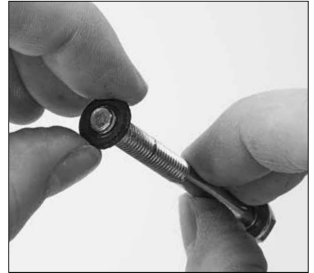
1.26 Replace plunger retainer gasket with new one from seal kit and apply a lubricant to the outside surface.
