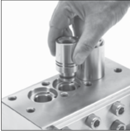
3.8 Remove V/P cylinders from IMDM.
