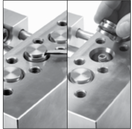
1.2 Use a flat tip screwdriver to remove valve plugs from each valve chamber.
