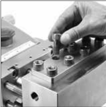
1.11 Apply anti-sieze lubricant (PN 6119) to threads of all eight (8) HSH screws and hand tighten.
