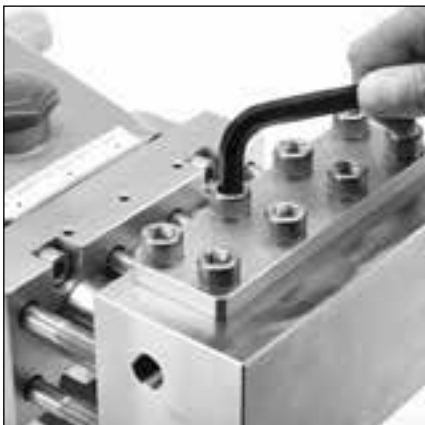
1.12 Use a M10 Allen Wrench to torque all eight (8) HSH screws to 398 in lbs, 33 ft lbs or 45 Nm in sequence show.
