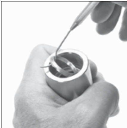
3.11 Remove male adapter from each V/P cylinder.
