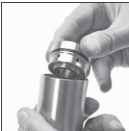
3.20 Lubricate seal case o-ring and inside diameter of each outer cylinder. Hand press each seal case assembly with low pressure seal facing outwards into outer cylinder.
