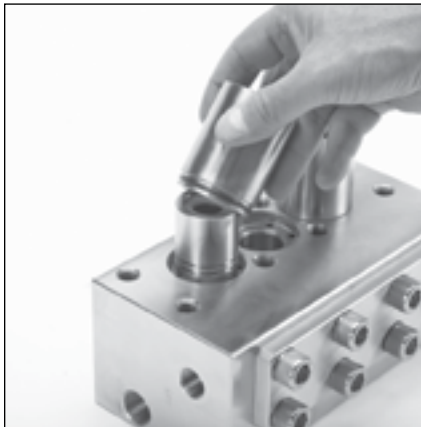
3.18 Lubricate and install o-ring into groove of each outer cylinder. Slide outer cylinder over each V/P cylinder and hand press into IMDM.
