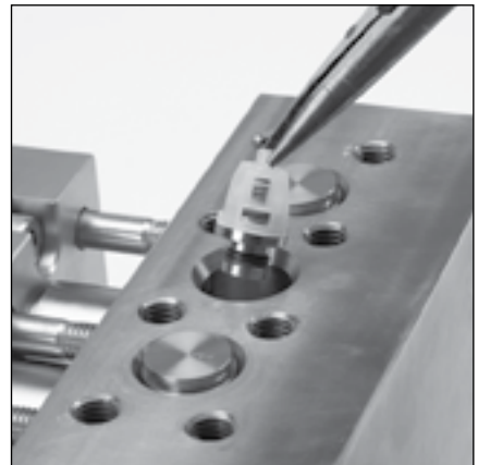
1.5 Use a needle nose pliers to grab the tip end of the spring retainer and pull valve assembly from each valve chamber.
