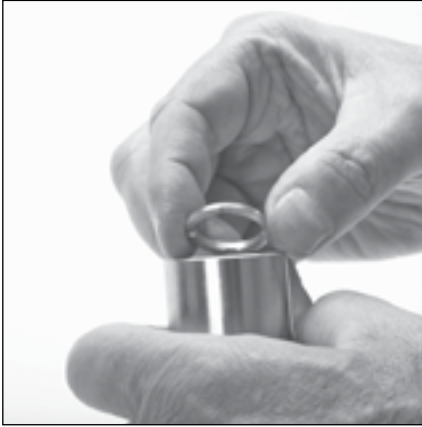
3.14 Install brass male adapter with flat surface down into each V/P cylinder.
