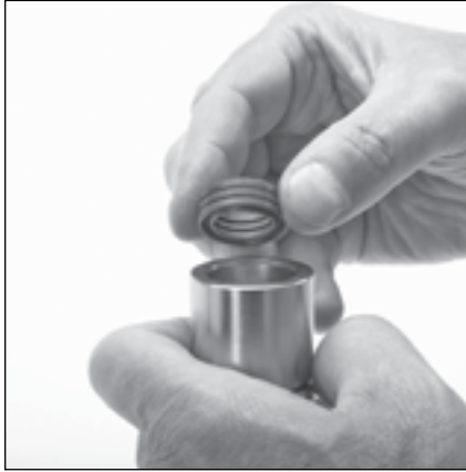
3.15 Lubricate and install v-packings with v-grooved side down into each V/P cylinder. Each cylinder requires three (3) v-packings.
