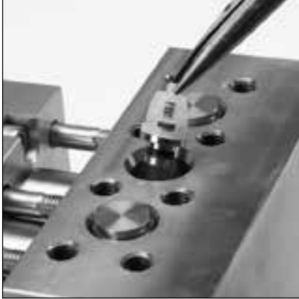
1.7 Place new assembled discharge valve assembly into each valve chamber.
