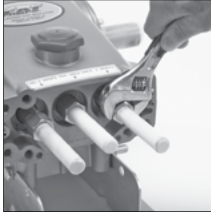
4.5 Use a 7/8" wrench to torque the three (3) plunger assemblies to 398 in lbs, 33 ft lbs or 45 Nm.
