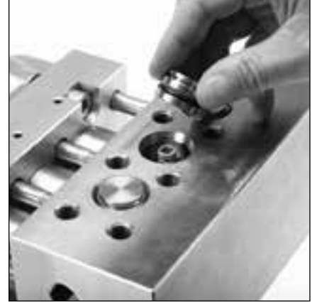
1.9 Press in valve plug into each valve chamber.
