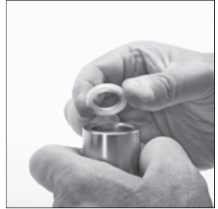
3.16 Install female adapter with v-grooved side facing down into each V/P cylinder.
