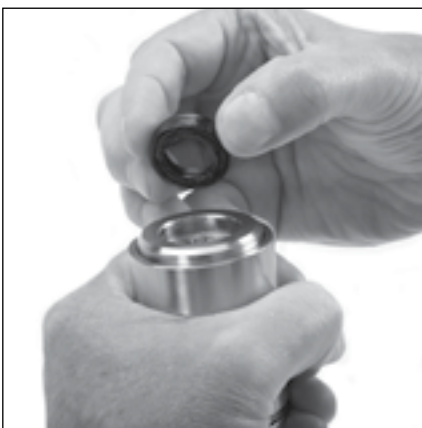
3.19 Lubricate outside diameter of each low pressure seal and inside diameter of each seal case. Install low pressure seal with spring side down into each seal case.
