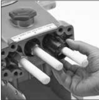
4.1 Remove seal retainers from crankcase.
