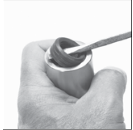
3.10 Remove v-packings (qty 3) from each V/P cylinder.
