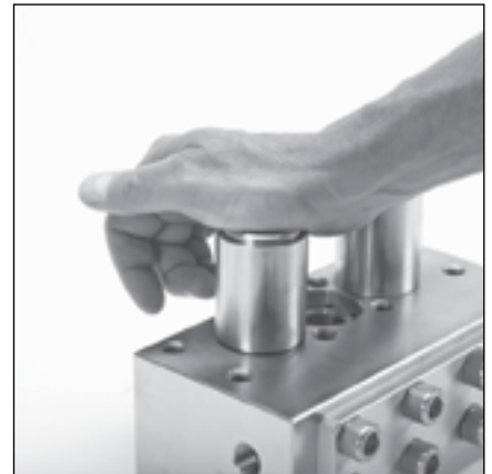
3.18 Lubricate and install o-ring into groove of each outer cylinder. Slide outer cylinder over each V/P cylinder and hand press into IMDM.
