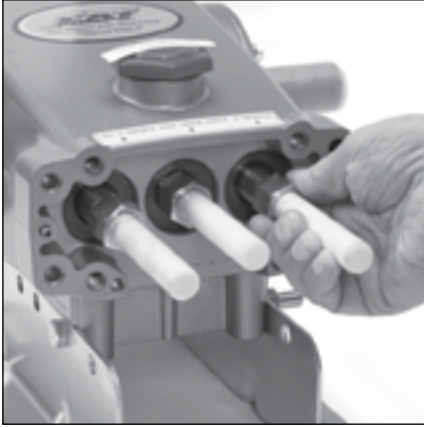
4.4 Install plunger assembly onto each plunger rod.
