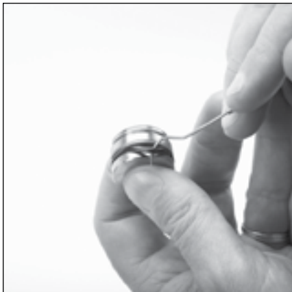
1.3 Use a pick tool to remove backup-ring and o-ring from each valve plug.
