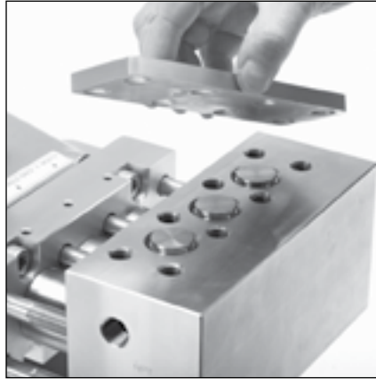
1.1 Remove valve cover.
